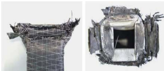
Figure 12. Failure of square hollow section steel tube [29].
